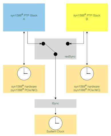
Figure 2: redSync for redundant System Clock Synchronization
