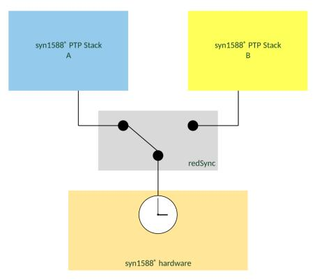
Figure 1: redSync for redundant Hardware Clock Synchronization
