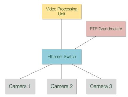
Figure 5: Industrial camera system with dedicated PTP Grandmaster
