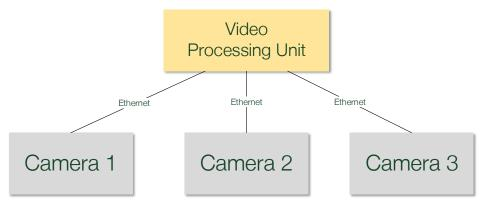
Figure 2: Industrial camera system with directly attached cameras
