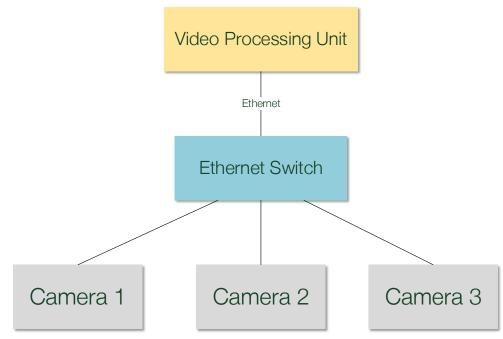
Figure 1: Typical industrial camera system
