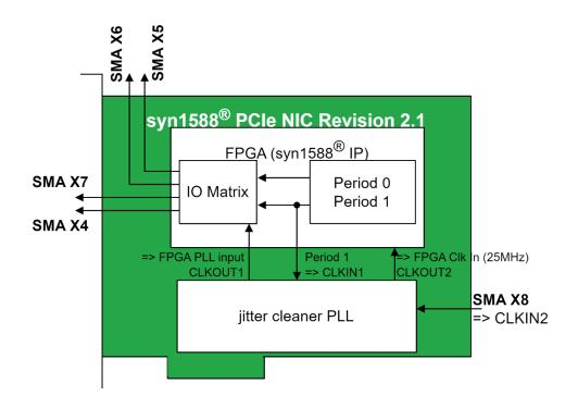
Figure 4: syn1588<sup>®</sup> PCIe NIC Rev 2.1 & 2.3 SMA connectors
