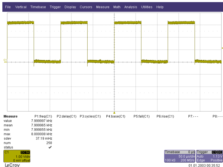
Figure 2 digital 8 kHz clock signal generated on connector X4
