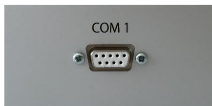
Figure 7 serial interface connector for the 19" rack-mount case
