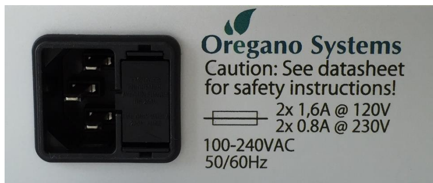
Figure 8 Mains connector with fuse drawer
