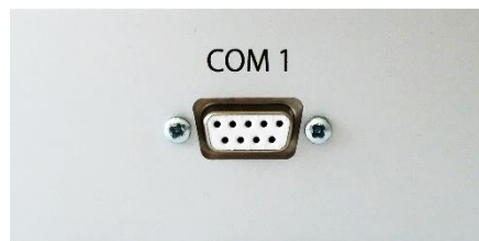
Figure 7 serial interface connector for the 19" rack-mount case
