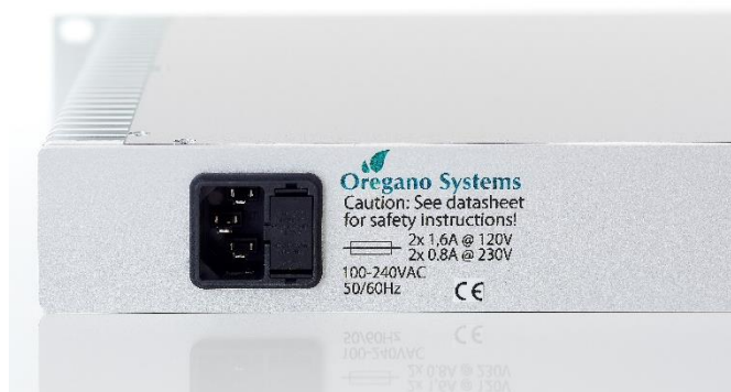
Figure 8 Mains connector with fuse drawer
