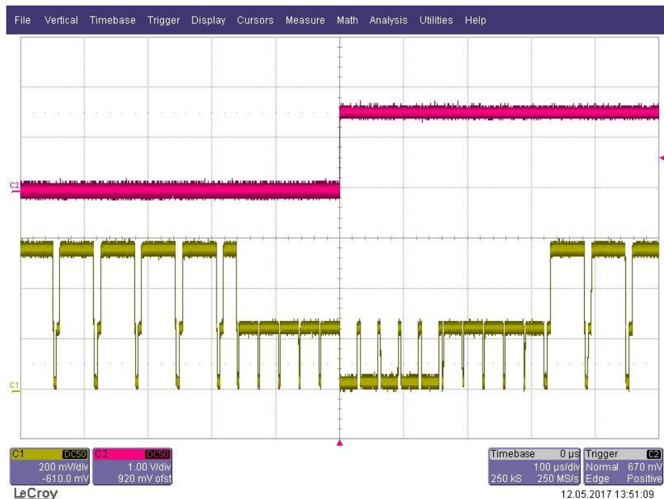
Figure 6 Analog Video Mode 625i (master operation)
