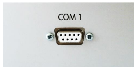
Figure 7 serial interface connector for the 19" rack-mount case
